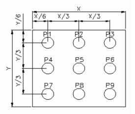
(Effective spatial Distribution) Hole Diameterø3mm ; 1 to 9 per Position Measured Luminous
